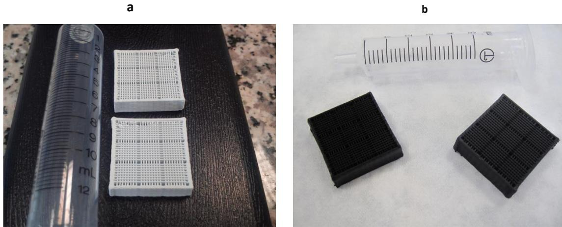
Figure 2. Optical image of 3D porous scaffolds produced by robocasting from (a) 45S5 bioglass ink and (b) 45S5 bioglass/graphene ink.
