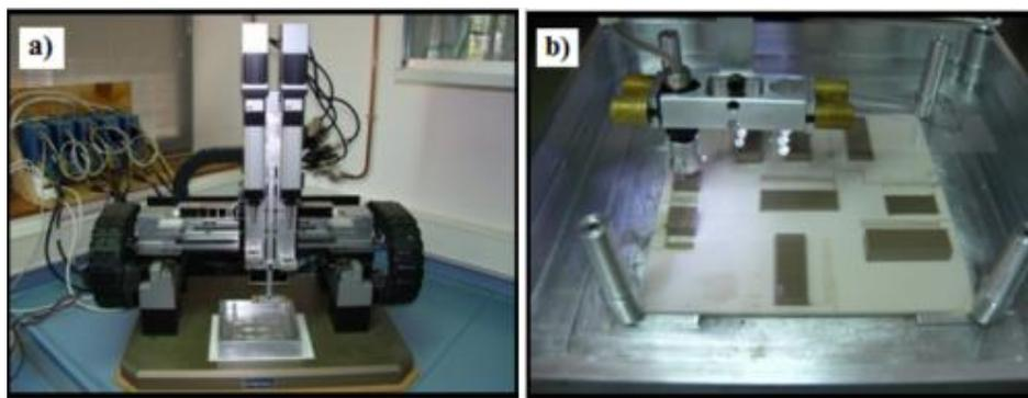
Figure 1. Optical images of (a) the robocasting system, (b) 3D robocast structures as-deposited within an oil bath.
